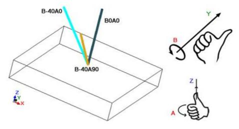
In a setup working that assigns the tool orientation, the XYZ coordinates are significant with respect to the nonoriented setup case.
