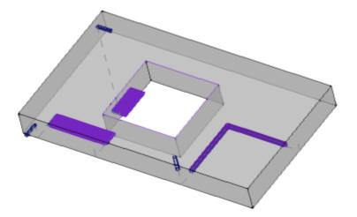
**Trim the overall dimension at the length of the tool**: it shows the overall dimensions for the segments considered **not over the piece** only (see previous point) and with an extension of the vertical overall dimension that is equal to the length of the tool. The picture shows the same overall dimension for all the segments not over the piece corresponding to the tool length of each profile.
