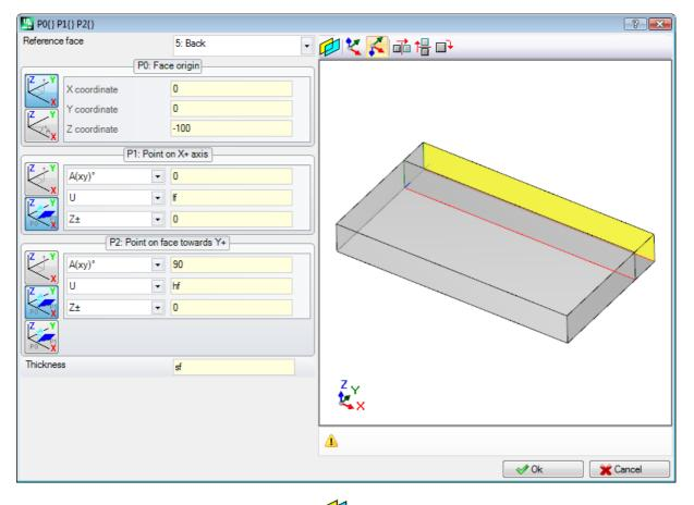
**Reference face:** Face 5: press then the button  $\checkmark$ . Set the Z coordinate of the P0 point to the -100 height to translate the face along the Z- axis of the reference face so as to obtain the face shown in the figure. If it is necessary, move the P0 point on the x and/or y coordinates: assign values different from 0; if it is necessary assign different length and/or height dimensions: replace If and/or h values.
