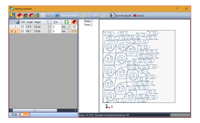
The solution can lead to more than one TCN program being generated: in the figure two. You can generate new solutions, as reported for the previous tool, and choose the solution to be applied.
