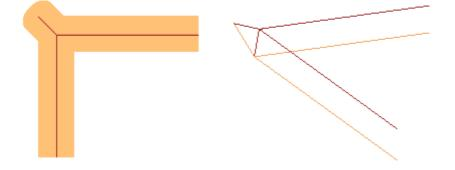
As clearly shown in figure, the rise on the corner is added to the "external part" of the profile. In a rectangular profile, finding the external part could not be more clear, but it is not always the case. A profile can show concave and convex parts and can be closed or not. For all these reasons, four possible options are associated to the **Sharp corner cut** field as follows:
