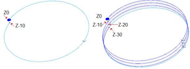
On the left: the original profile, assigned with a circle carried out with a Z depth from 0.0 to - 10.0. On the right: the profile as modified by the tool by the application of the following assignments:
