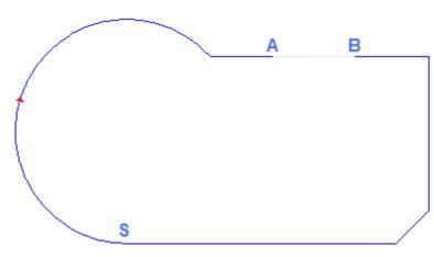
On the profile 2 cut points have been marked and namely: (A) and (B) (the two points can lie on the same segment or on different segments). The part of profile between the two points is deleted (**ATTENTION**: in the direction of the original direction).
