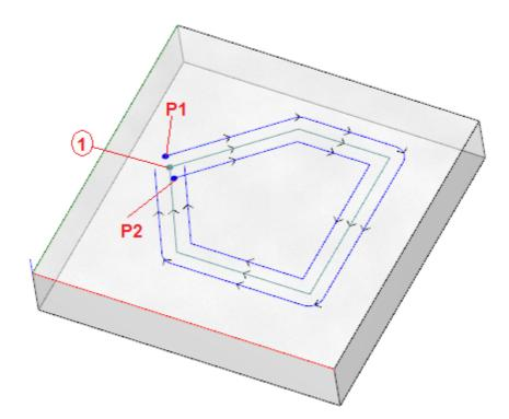
The central profile corresponds to the programmed profile: the setup is indicated as a point (1); (P1) shows the setup of the profile taken through left Compensation;
