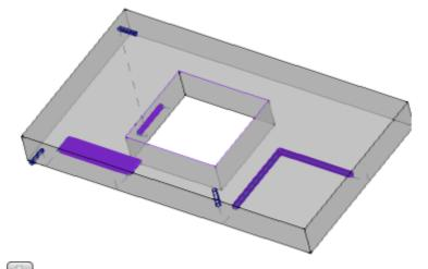
**Trim the overall dimension at the piece**: it shows the overall dimensions of the segments considered **not over the piece** only (see previous point) and with an extension of the vertical overall dimensions that is restricted to the intersection to the piece (original parallelepiped) and anyway not greater than the length of the tool. In case of curved face or surface, the vertical overall dimension interprets as: **Trim the overall dimension at the plane of the face**.
