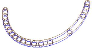
The full segment view can be particularly useful in case of emptying profiles, in order to estimate the real removal of material. The figure makes the difference between the two representations clear.
