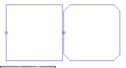
On the left a rectangle with corners. On the right the final result after the tool application to the whole profile.
