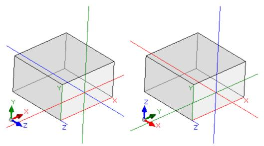
[on the left] both the entries are disabled: Show the local three points and cursor to the face; [on the right] both the entries are enabled: Show the absolute three points and cursor on the face. • **Customize the colour or pattern of the panel**: enables or disables the application of the current program of the colour or pattern, if assigned in *Special Settings* of the program. The default is not enabled, and the voice may not be visible to the assignment.
