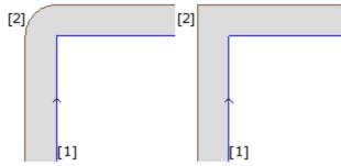
In the left figure the compensated profile moves around the original corner with a radius arc equal to the tool radius; in the figure on the right, the compensated profile continues up to the external intersection point of compensated linear segments.
