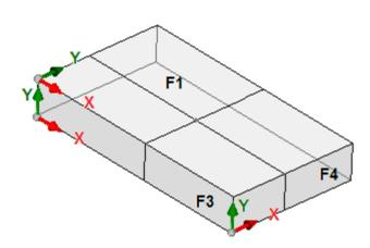
It is necessary to adjust the application point for induced calls as X and/or Y axes could not correspond between different faces. Let us consider this figure (three visible faces of piece are shown)
