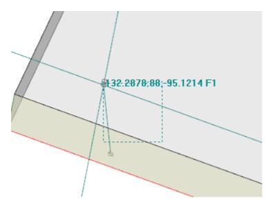
the hatched area shows the dimension according to which the graphic searching area of the snap entity has been enlarged: we may indicate it as snap cross-hair. As already told, the searching graphic area is restricted and starts from a minimum dimension of some pixels and it is enlarged - always to a maximum area - until a correspondence is found (see also: Customize TpaCAD -> Views -> Mouse).
