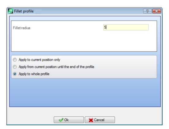
• Fillet radius: radius of the fillet arc inserted on the corner.
