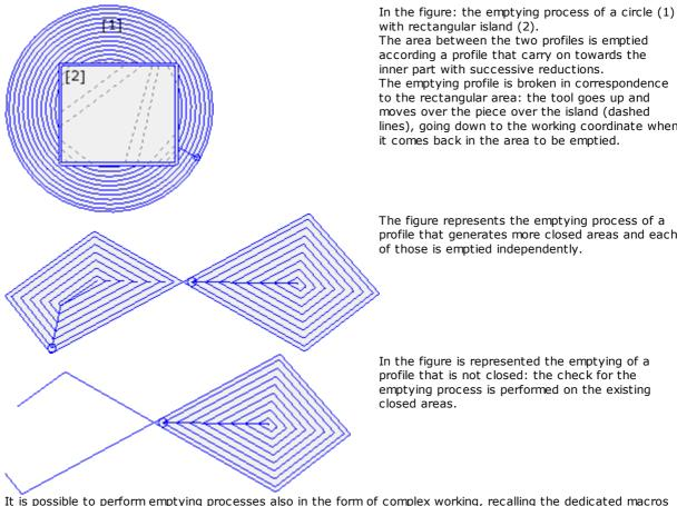
to the rectangular area: the tool goes up and moves over the piece over the island (dashed lines), going down to the working coordinate when it comes back in the area to be emptied.
