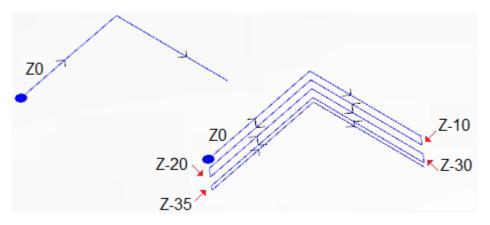
On the left you will see the original profile, assigned with two linear segments carried out at a depth measure of Z = 0.
