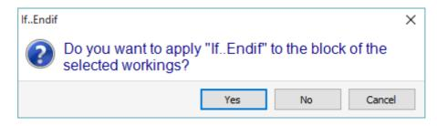
Choose **[Yes]** to insert directly into the block the group of the selections of which the current working is part. In the case as above (Insert If.. Endif), being on the line 5 and having selected the lines from 3 to 12:
