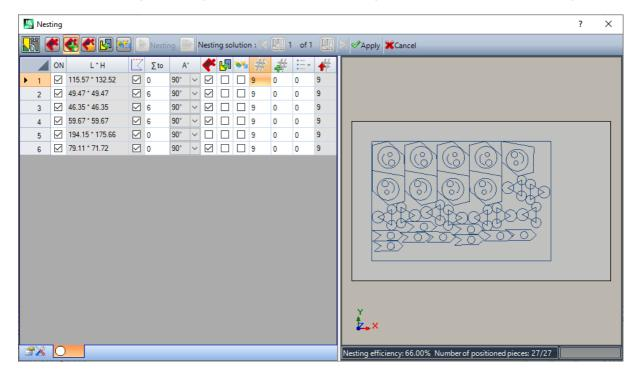
The figure shows the rectangle assigned for the placement of the profiles.
