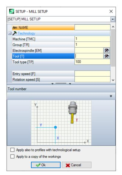
In the window above, the setup code to be assigned is first selected in the window among those in the list (in figure: [SETUP] MILL SETUP) and the list of parameters is updated with the data related to the selected working. Then, set the technological parameters and the working properties and confirm by pressing **[OK]** to apply the assignment.
