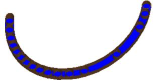
**Overall dimension of the profiles with linear segment**: the profiles are represented with a thickness equal to the tool extent but with a non-full profile. In the figure the external contours of the extents are displayed. This selection excludes the representation of edge points and direction arrows.
