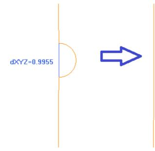
On the left the original path is displayed, light-coloured; it is clear that the indented area and the blue segment highlight its scale that is less than 1 mm;
