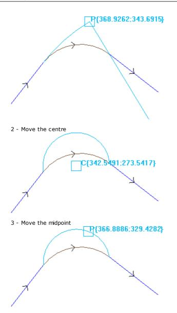
If the segment is a **conic arc (ellipse)** it is possible to change the length of the segment, expressed as linear or angular length:
