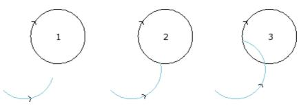
The arc represents the segment which must be extended up to the point of intersection with the circle
