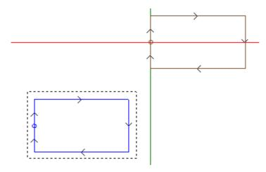
The rectangle selected in figure represents the subroutine development (a rectangle crossed clockwise, with start point located in the middle of the left vertical side). The cross cursor indicates the application point P1: subroutine start point is located in P1 (rectangle setup).
