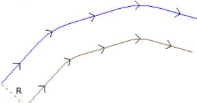
The original profile is outside. The compensated profile is inside, so the required **Compensation side** is **Right**. **R** represents the compensation radius.
