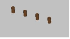
The drawing shows a 3D impersonation example of point workings (or isolated setups), that have an overall dimensions view: for each working is represented a little cylinder that is as high as the programmed depth. The little cylinder fill is determined by the selection **Show extent of points and setups with full segment**. The default setting is disabled.
