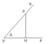
The user should remember that an angle is defined as positive when it rotates in counterclockwise direction. Let us consider an angle (A): (in radiants) of vertex V and sides a and b. Let us take on the half-line b any point P distinct from the vertex V. Let us project it on the half-line a: be H the point of the perpendicular described by P on a.
