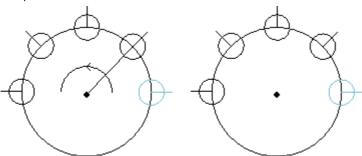
Repetition of the working marked with a bold line for **5** elements, angle to fill up: **180°**, counterclockwise rotation. The left figure shows the series whose **Rotate item in the series** field is not selected.
