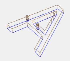
The drawing shows a 3D representation example of profiles, with the overall dimensions view enabled: each profile segment underlines the tool overall dimension in the piece. The default is disabled. The application of the selection is conditioned by the entry state **Overall dimensions in 3D graphs**, in View on menu. The value of the selection can be changed from the local menu, managed on **Overall view in 3D graphs**, in the View on menu.
