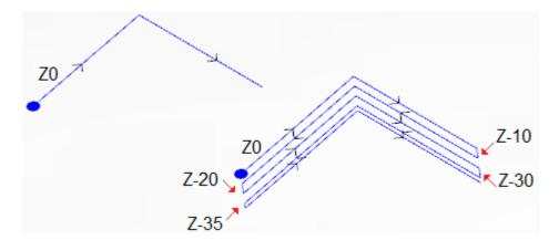
On the left you will see the original profile, assigned with two linear segments carried out at a depth measure of Z = 0.
