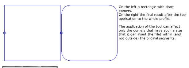
It is possible to generate profiles by inserting some junction arcs into the corner points of the profile, also in the form of complex working, by recalling the Programmed tools in the list of the workings. In the group of TOOLS select the STOOL: FILLET PROFILE:
