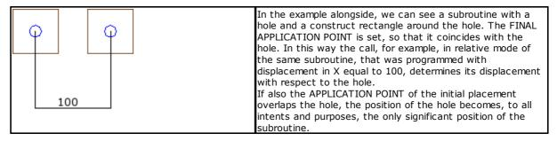
The use of the instruction FINAL APPLICATION POINT excludes the possibility of hooking the subroutine after the working and recognizing the profile continuation.
