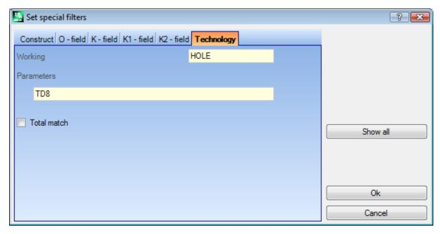
According to the data set in the example window, only the workings with ASCII code "HOLE" and TD parameter set to value 8 are displayed.
