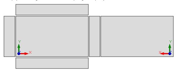
• **Vertical development**: the panel is exploded with vertical development (if the face 2 is assigned, it is displayed below with the vertical opening of the panel).
