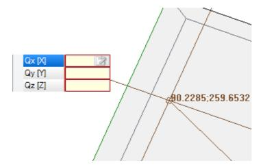
• significant assignment of only one coordinate (abscissa or ordinate): on the working area, only one corresponding field is marked and a horizontal or vertical cursor highlights its meaning.
