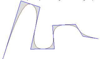
From the same profile by selecting the option **Cubic B-spline** we get the curve:
