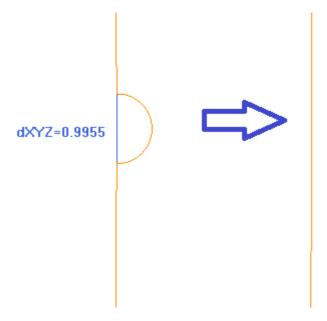
On the left the original path is displayed, light-coloured; it is clear that the indented area and the blue segment highlight its scale that is less than 1 mm;
