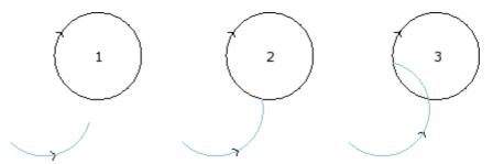
The arc represents the segment which must be extended up to the point of intersection with the circle
