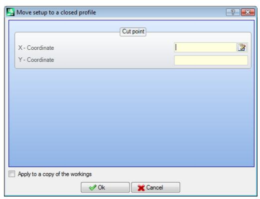
**X - Coordinate, Y - Coordinate**: they set the setup new position. Click the icon to select with the mouse in the graphic area. Acquiring with the mouse the position of the point, the coordinates are assigned so that they correspond to a point along the profile. If the same coordinates have to be directly assigned or modified, the nearest point to the point set along the profile is searched.
