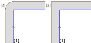
In the left figure the compensated profile moves around the original corner with a radius arc equal to the tool radius; in the figure on the right, the compensated profile continues up to the external intersection point of compensated linear segments.
