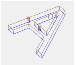
The drawing shows a 3D representation example of profiles, with the overall dimensions view enabled: each profile segment underlines the tool overall dimension in the piece. The default is disabled.
