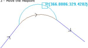
If the segment is a conic arc (ellipse) it is possible to change the length of the segment, expressed as linear or angular length:
