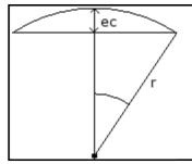
The figure shows the geometric meaning that has been given to the chordal error set (a set value of chordal error can be 0,05 mm).
