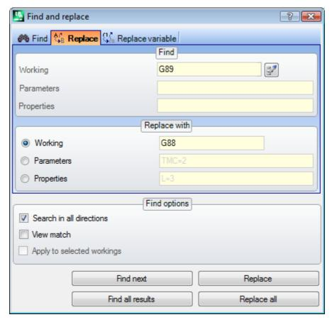
Suppose to open a program which uses invalid working codes in the current program configuration (in the example: "G89" does not match any working operating code).
