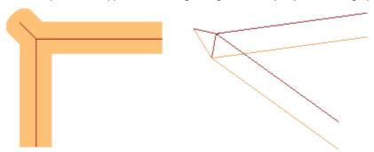
As clearly shown in figure, the rise on the corner is added to the "external part" of the profile. In a rectangular profile, finding the external part could not be more clear, but it is not always the case. A profile can show concave and convex parts and can be closed or not. For all these reasons, four possible options are associated to the **Sharp corner cut** field as follows:
