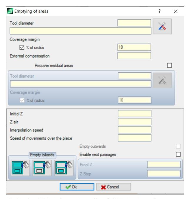
A closed area is emptied when inside an area is generated a profile that is made up by successive passes obtained with progressive deviation from the original profile, until the internal area is fully covered. If required, the emptying process guarantees the observance of internal closed areas (islands) and it tries to recover the not fully emptied areas, because of the original observance of the original area limits.
