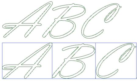
The text developed on the top applies a *metric* spacing. The text developed below applies a *geometric* spacing: around each character its own overall rectangle is shown.
