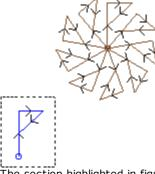
The section highlighted in figure corresponds to the single element as programmed in the subroutine. All repetitions are applied to the base application point and rotated to complete the round angle.
