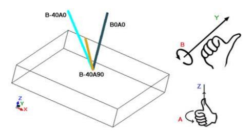
In a setup working that assigns the tool orientation, the XYZ coordinates are significant with respect to the non-oriented setup case.
