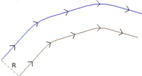
The original profile is outside. The compensated profile is inside, so the required **Compensation side** is **Right**.
