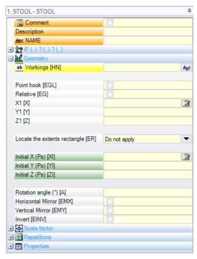
The working is similar to the subroutine application SUB code. Now the Workings field replaces the subroutine selection field.
