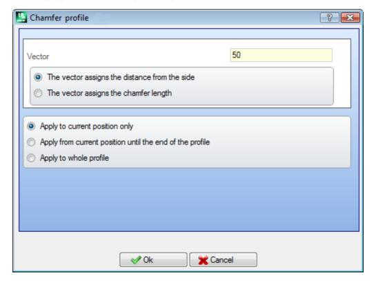
• Vector: the assigned length to define the chamfer.
