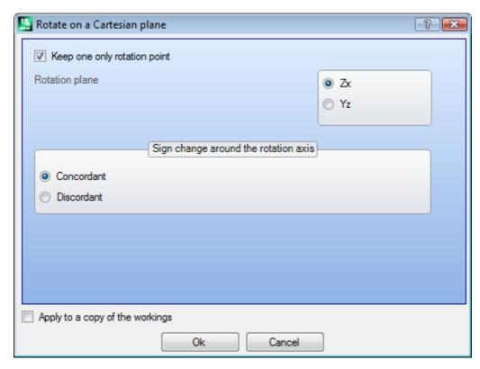
This tool rotates the profiles(s) of 90° around one of the two coordinated axes of the face plane. The possible2 options are:
