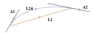
${f L1}$  is the linear segment that joins the extreme points of the segment (the segment is the comparison term with the generated curve).
