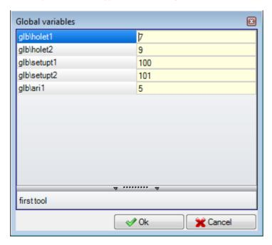
The table can show no more than 300 numeric variables, that can be recalled by symbolic name only, with the following format: "glb\xxx" with "xxx" = symbolic name. The variables are assigned in TpaCAD configuration and can be used for each setting.
