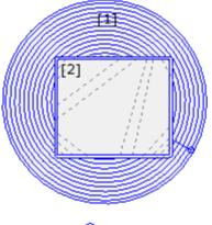
In the figure: the emptying process of a circle (1) with rectangular island (2).
