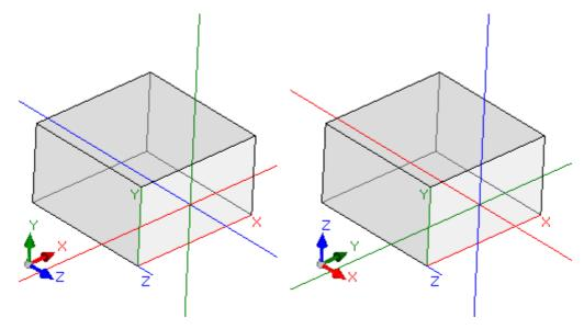
[on the left] both the entries are disabled: Show the local three points and cursor to the face; [on the right] both the entries are enabled: Show the absolute three points and cursor on the face.
