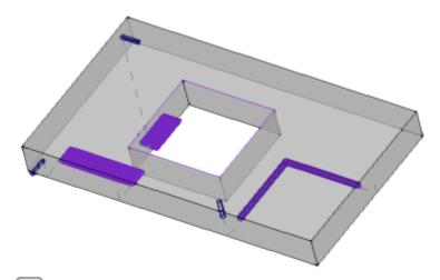
Trim the overall dimension at the length of the tool: it shows the overall dimensions for the segments considered **not over the piece** only (see previous point) and with an extension of the vertical overall dimension that is equal to the length of the tool. The picture shows the same overall dimension for all the segments not over the piece corresponding to the tool length of each profile.
