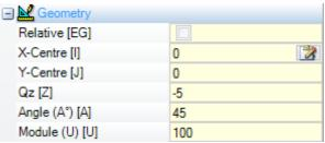
The figure shows the polar coordinates. The Z coordinate is directly assigned, as in the case of assignment with Cartesian coordinates. The position of the point in the XY plane is specified by giving its distance from a centre and its angle (in degrees) in XY plan from X axis. In the figure:
