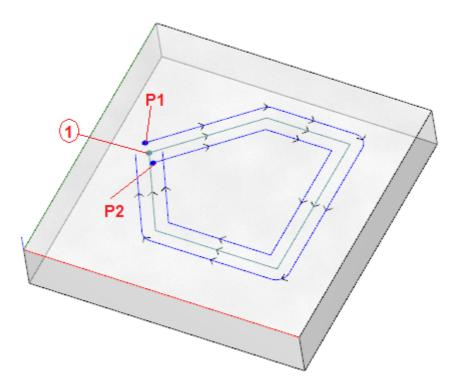
The central profile corresponds to the programmed profile: the setup is indicated as a point (1); (P1) shows the setup of the profile taken through left Compensation;
