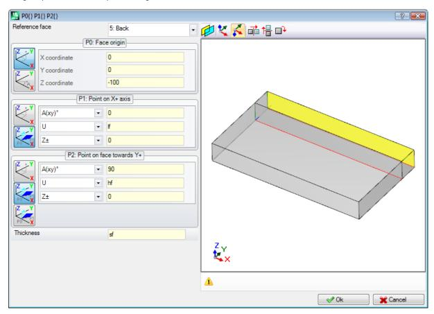
Reference face: Face 5: press then the button  $\cdot$ . Set the Z coordinate of the P0 point to the -100 height to translate the face along the Z- axis of the reference face so as to obtain the face shown in the figure. If it is necessary, move the P0 point on the x and/or y coordinates: assign values different from 0; if it is necessary assign different length and/or height dimensions: replace If and/or hy values.
