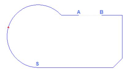
On the profile 2 cut points have been marked and namely: (A) and (B) (the two points can lie on the same segment or on different segments). The part of profile between the two points is deleted (**ATTENTION**: in the direction of the original direction).
