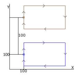
The figure corresponds to two applications of the subroutine in the example (making a rectangle):
