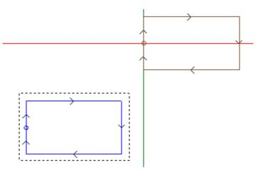
The rectangle selected in figure represents the subroutine development (a rectangle crossed clockwise, with start point located in the middle of the left vertical side).
