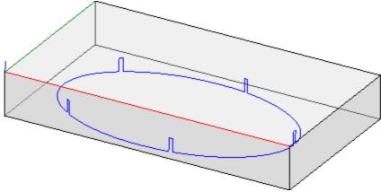
By applying the interruptions, it is typical to use the tool with cut technologies that differ from a traditional tool: plasma/laser cutting or similar.
