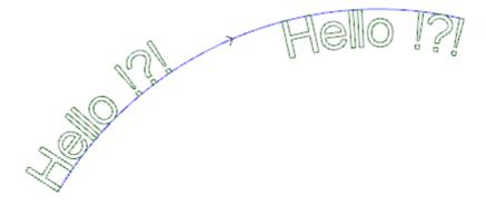
The Figure above shows an example of generation of 2 equal writings, with selection of no automatic text distribution along a circular segment in clockwise direction.
