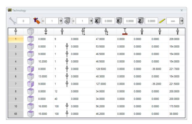
If the universal tool management is enabled in the TpaCAD Configuration, the first page shows the list of universal tools and the machine and group fields have a value of 0.
