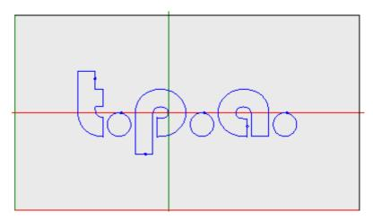
The figure is an example of face graphics. We can also see the cross-cursor full-field on the view. The reference system origin and the face axes are indicated.
