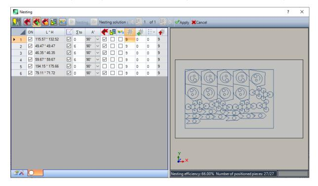
The figure shows the rectangle assigned for the placement of the profiles. For each group we have performed the placement of 9 copies for a total amount of 27/27 placements required.
