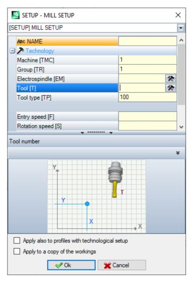
In the window above, the setup code to be assigned is first selected in the window among those in the list (in figure: [SETUP] MILL SETUP) and the list of parameters is updated with the data related to the selected working. Then, set the technological parameters and the working properties and confirm by pressing **[OK]** to apply the assignment.
