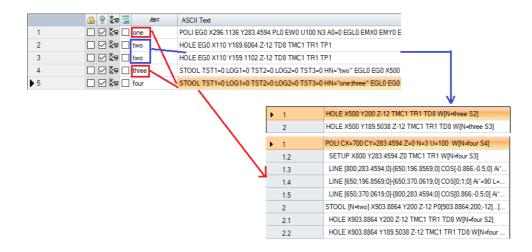
The line 4 is a STOOL code that is applied to the workings called "two" (HOLE workings of line 2 and 3):
