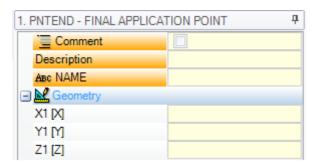
The three fields of X1, Y1, Z1 set the final application point, that does not necessarily need to coincide with the coordinates of a working point. The programming of the coordinates occurs in absolute mode and for the coordinates, that were not set, the value 0.0 is taken up.
