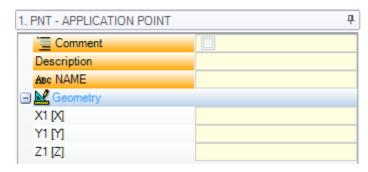
The three fields X1, Y1, Z1 assign the point to be located, when the subroutine itself is recalled.
