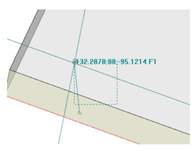
the hatched area shows the dimension according to which the graphic searching area of the snap entity has been enlarged: we may indicate it as snap cross-hair. As already told, the searching graphic area is restricted and starts from a minimum dimension of some pixels and it is enlarged - always to a maximum area - until a correspondence is found (see also: Customize TpaCAD -> Views -> Mouse).
