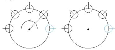
Repetition of the working marked with a bold line for **5** elements, angle to fill up: **180°**, counterclockwise rotation. The left figure shows the series whose
